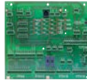
■ JUNCTION BOX MODULE
