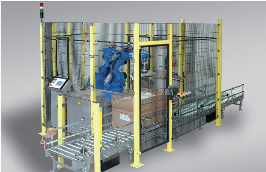
**Robot-supported plant systems are widespread in production and packaging. Their working area must be separated from that of the operator – usually by a safety fence. (Photo: ETT Verpackungstechnik)**
