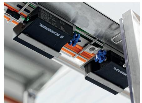
Also at the field level – the figure shows a safety interlock on the guard door for a packaging machine – flexibility is required.
