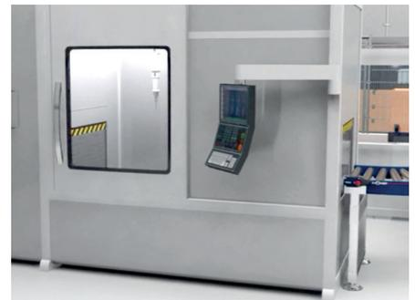
**01 On large machine tools, not only the safety doors but also the locking bolt of the solenoid interlock are actuated electrically**
