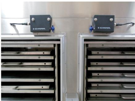
**02 Both doors of the cooling cells are held closed by AZM 300 units respectively while the blood plasma is shock frozen by means of contact cooling**
