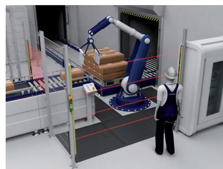
**To make the danger zones and hazard areas safe, optoelectronic safety devices are often a wise option – as an alternative to a safety door**
