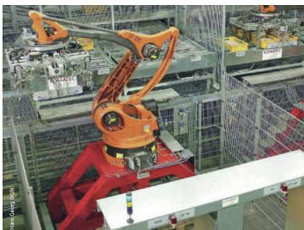
**Robot-supported plant systems are widespread in production and packaging. Its working area must be separated from that of the operator – usually by a safety fence**
