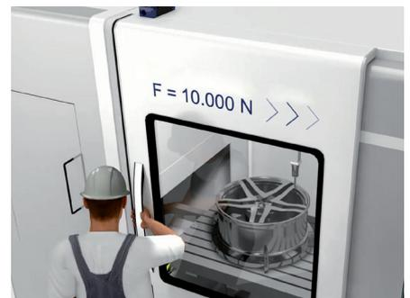
**02 The locking bolt of the solenoid interlock is capable of a holding force of 10 000 N**
