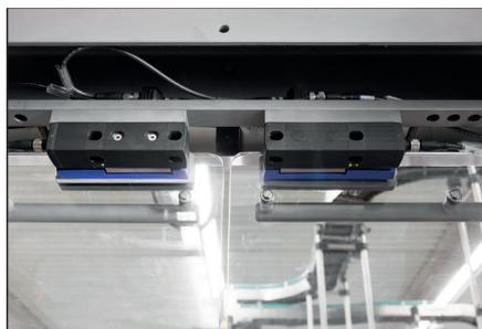
**On the feeding machine of the Optima MPS, the MZM 100 from Schmersal was used to secure rotatable safety guards.**
