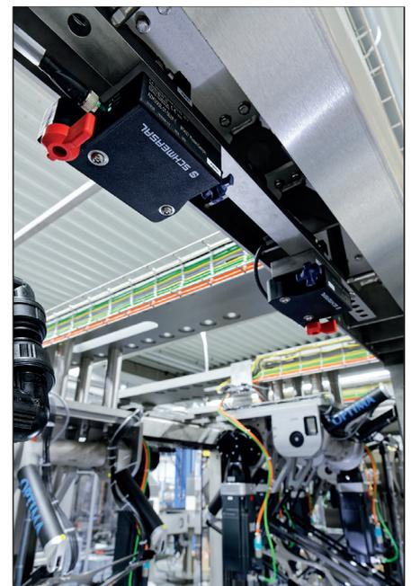
**The new Optima MPS (Multi Packaging System) is equipped with the solenoid interlock AZM 300 to provide personal protection especially for the accessible areas of the machine. The emergency release enables people, who were accidentally trapped in the danger zone to quickly leave the area.**
