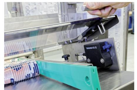
Securing the magazine in which the preformed cups are located
