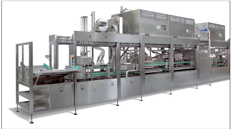
**The Combiseptic 81 filling and sealing machine achieves an output of up to 16,000 cups per hour at the Valio dairy company in Finland**
