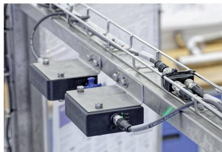
Two AZM 300s for securing two rotatable safety guards with SD bus connection
