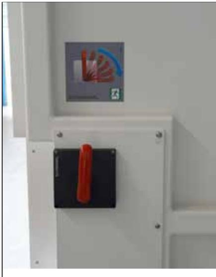
**Image 3 (sijenoptik 4):** With the panic handle, a trapped person can leave the hazardous area even when the solenoid interlock is closed
