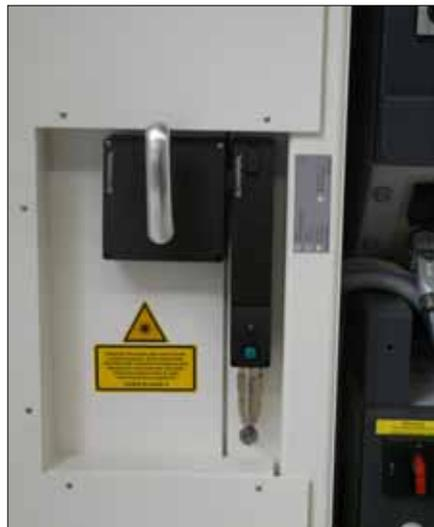
**Image 4 (sijenoptik 1):** For Jenoptik, Schmersal developed a variant of the AZM 200, which detects the position "Safety guard ajar/closed, but not locked".
