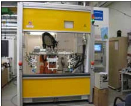
**Image 1 (sijenoptik-Votan-A-compact):** A worldwide applied specialty of Jenoptik Automatisierungstechnik GmbH: laser plants, which generate invisible seams for vehicle airbags. The image shows a plant in the production line at Jena shortly before its completion.
