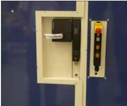
**Image 6 (sijenoptik 14):** The combination of AZM 200 and BDF 200 provides for a smooth configuration of ergonomic man-machine interface at the safety guard.
